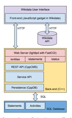
Figure 6: *Primary Sources Tool* architecture. The front-end (JavaScript) sends HTTP requests to the back-end (C++) to retrieve and update entities or statements, stored in a relational database. Approved statements are in addition written by the front-end to the Wikidata REST API.
